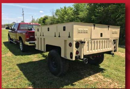
Above: RUGGED RIAB can be towed by standard GSA trucks with additional 12V adapter kit. TLDs charge inside trailer when plugged into 120VAC power via supplied power cable or Portable Quiet Generator option.
