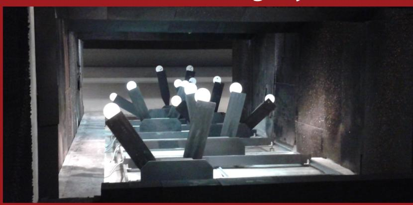
Strategic Systems' Reactive Steel Range is a computer controlled target system for live-fire training. The system uses compressed air to raise and lower AR500 steel head-plate targets. The Reactive Steel range system gives Range Supervisors great flexibility in training by allowing them to change the position, timing and other training aspects very quickly.
