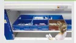
Side walls of the access opening are equipped with shelf rails, enabling the positioning of multiple trays in the access opening as well as individually ergonomically adjusted tray delivery heights for each operator depending on their physical height.
