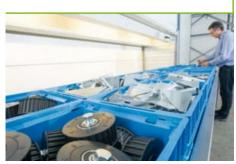
Uniquely powerful: Our heavy-duty tray can carry 1,763.7 lbs (800 kg) loads with an effective width of 159.4 in (4,050 mm), making it ideal for picking medium-heavy to heavy parts and setting new standards in terms of load capacity.
