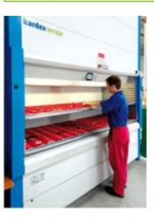
A dual tray delivery option makes it is possible to use two work levels in the access opening. A tray is delivered into the first work level in the access opening and the shutter door closes. While items are stored or removed, the next tray is being retrieved and kept in a waiting position behind the access opening, decreasing wait times.
