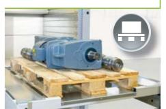
The "pallet handling" application ensures that pallets can be placed directly on the pallet trays by means of forklift or pallet truck and stored in the positioning facility. This saves floor space and reduces the need for high-rack stacker trucks. In addition, stored goods are found much more quickly. In summary, this application effectively helps to cut costs and raise productivity, and is also a plus from a safety perspective.
