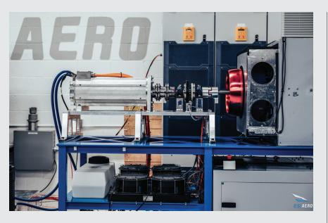
ORIGINALLY DESIGNED FOR THE DEVELOPMENT OF THE X-57 MAXWELL, this dynamometer is uniquely capable of characterization of hybrid and electric drivetrains for aircraft certification. The EDS200 is a stand-alone system essential for Advanced Air Mobility development. The EDS200 system also regenerates power from the test article, significantly reducing the energy consumed during testing.
