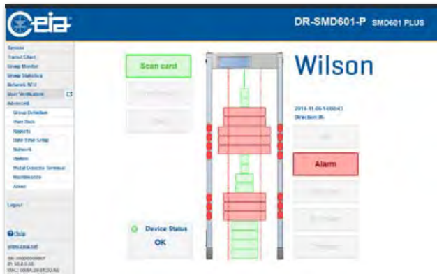
Each transit is compared with the individual's profile stored in the database.
